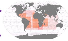
The multi-resolution modeling system along with the locations of various component models. The fine scale models (dark coral) are nested within the two basin scale obtains cale domains (light coral). The basin scale domains are in-turn nested within the 1/4\* global model (magenta).
